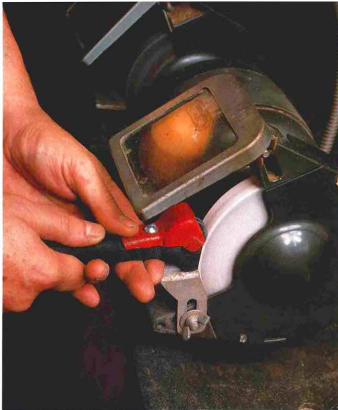
Norton's 60-grit wheel, off-white in color, with a variety of wheel dressers (shown counterclockwise from top): a star wheel, a single-point diamond, a Norbide stick and a plain abrasive stick.
