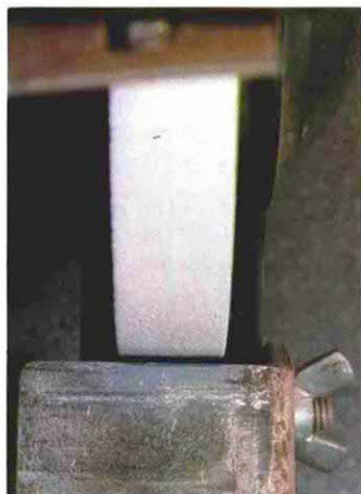
Bottom photos show Bay State's 100-grit wheel before and after dressing. At left, after much grinding of lathe tools, the wheel is worn concave with some embedded steel particles, which cause excess heat. Top photo shows the initial coarse dressing with a star wheel; center photo shows final truing with a Norbide stick.
