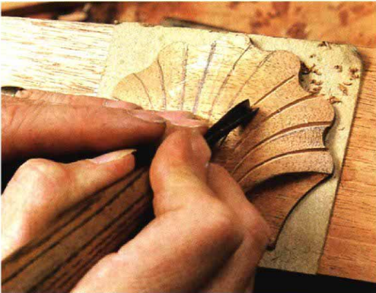
Pivot off your knuckle to control curves when drawing the rays (top). Define the rays with parting tool cuts (above). Adjust spacing by leaning the tool.
