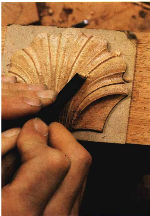
Shape tips of convex rays with a 1/2-in. #3 gouge, carefully avoiding tearout on cross-grain cuts (above). Left hand helps control the tool on concave rays (below).
