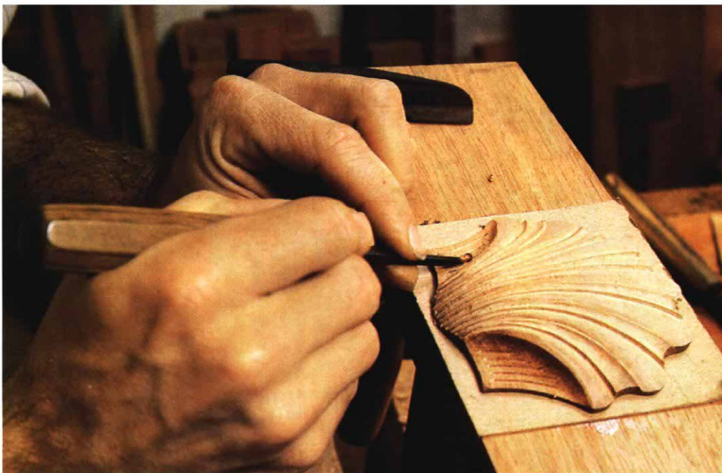
Cut from the bottom upward with a 1/8-in. #11 veiner to carve the veins in the wings.
