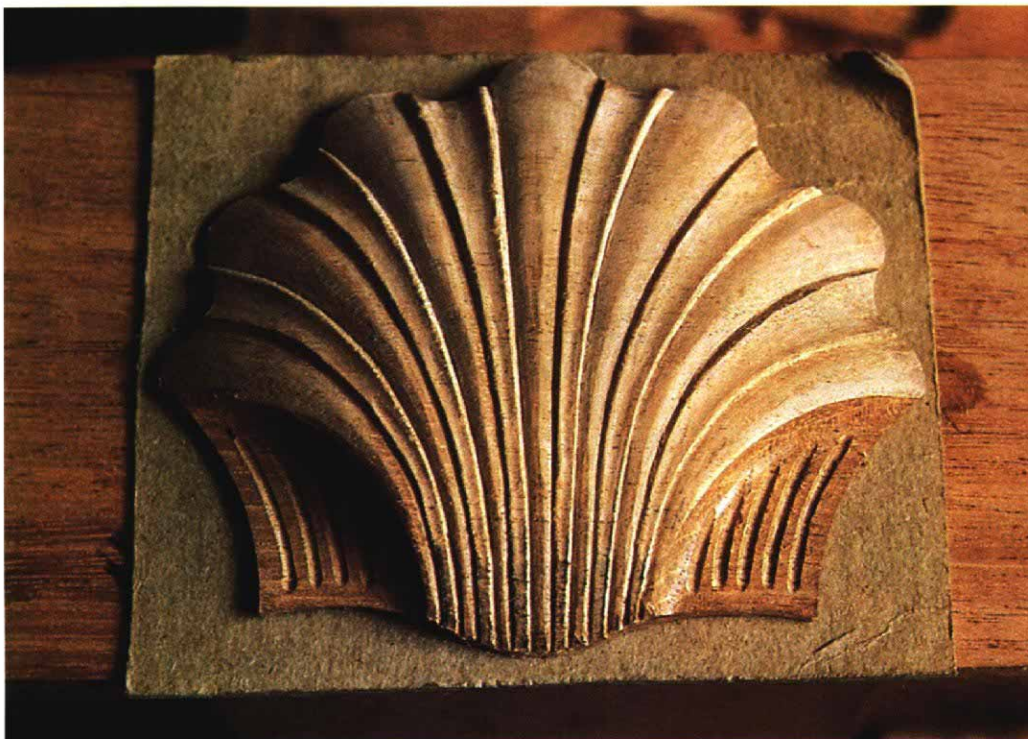
The finished shell is ready to be separated from its backing and glued on a piece of furniture. The curves and flats are designed to catch and play with light and shadow.
