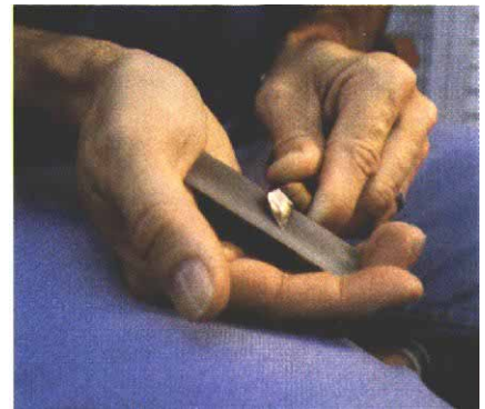
Sharpen the cutting knife at a 10° angle to the stone, as shown above. For a straight, smooth edge, always work on a stone that is large enough to hone the entire blade at once.
