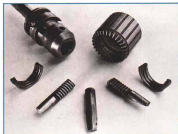
In the type A chuck (most Jacobs chucks are type A), the ring gear is part of the outer sleeve. A separate split nut works the jaws. Note that it's not necessary to remove a tapered spindle adapter to disassemble a chuck.
