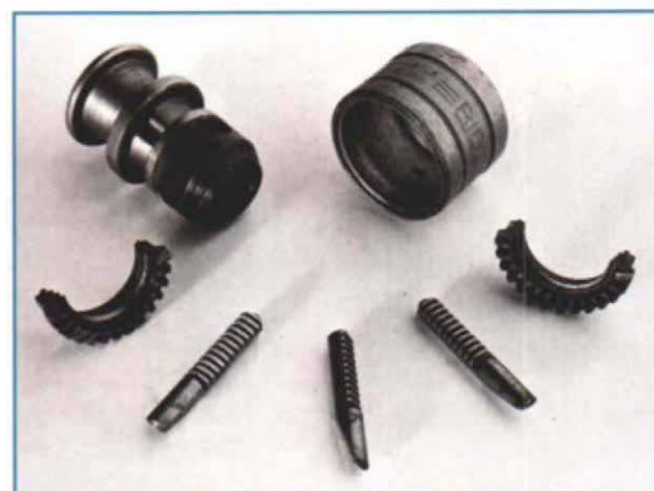
In the type B chuck, the ring gear is part of the split nut that works the jaws. Pressure must be directed against the narrow outer edge of the sleeve, not against the ring gear, to slide the sleeve off.
