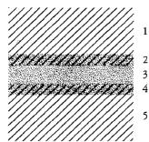
must "wet" the wood to establish molecular closeness for specific adhesion. Phase 3 is the adhesive itself, which holds together by cohesion.
