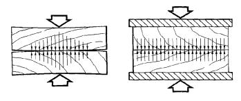
the middle of a flat board will not be evenly transmitted to its edges. It is therefore essential to use heavy wooden cover boards or rigid metal cauls to ensure proper distribution of pressure.
