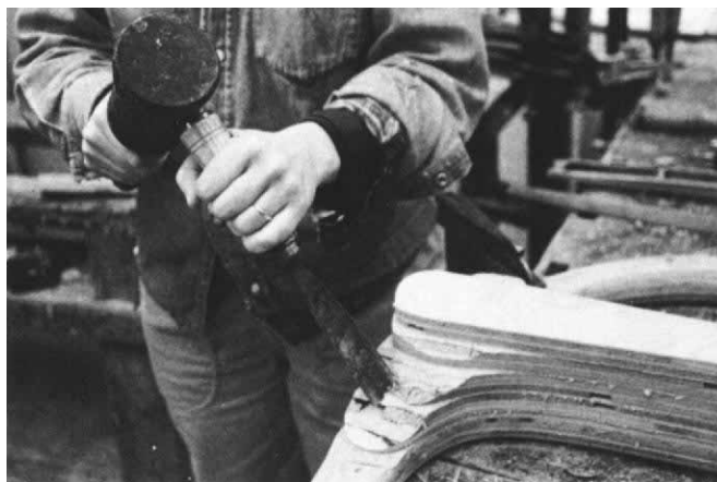
When side has been shaped and four layers added to start the seat, gouge and Surfform remove the stair-steps.
