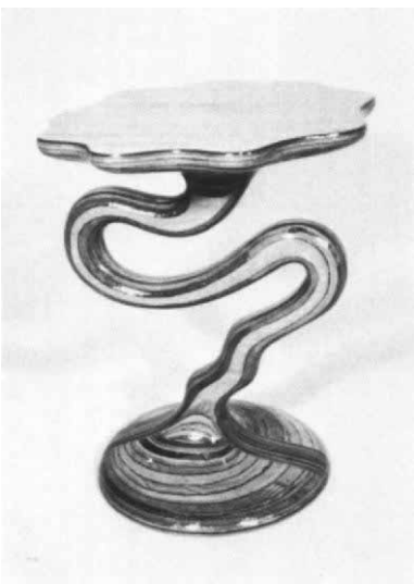
Sinuuous bend of three layers of plywood is made first; it is very strong and needs no reinforcement. Two small lozenges are glued and shaped for the transition atop the base, then the bottom plate is screwed on, and the half-layers of the base itself fit in between. Similarly the tabletop, except the surface piece hides the screws into the upright section.
