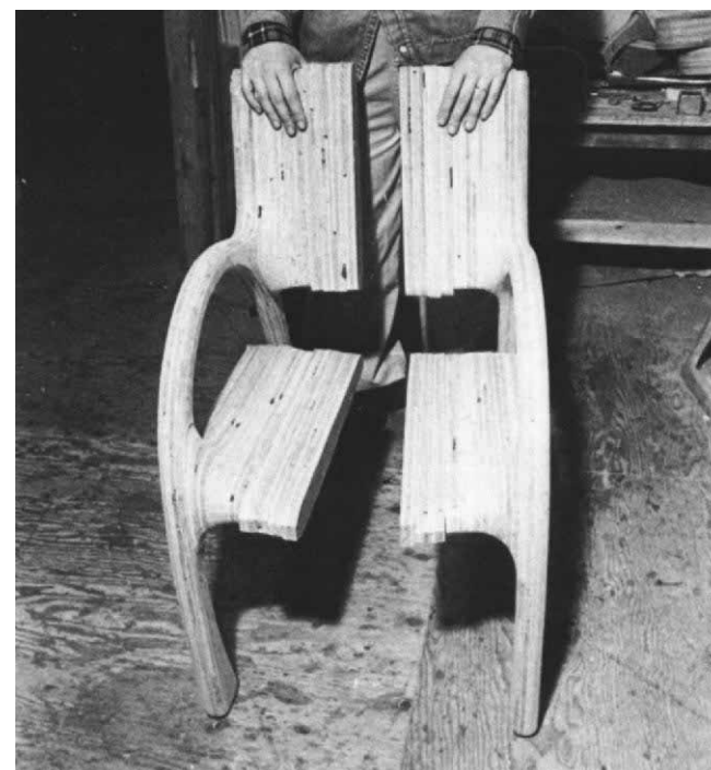
A wedge-shaped section will join the two halves, with dowels for reinforcement because the seat is supported only at the front.
