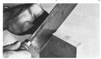
It is probably neater and easier to saw rather than to chisel the ends out. Clean up the corners between tails with a chisel before trying the joint.
