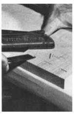
gauge line. This will establish a positive edge to line the chisel against. It will also lessen the chance of the chisel drifting back beyond the marking gauge line during chiseling. Now you are ready to take a heavier cut.
