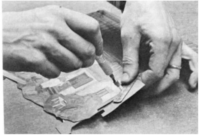
Sewing needle is used to make hole along line of cut. Jeweler's saw blade will then be fed through and mounted on the jig saw for cutting out.
