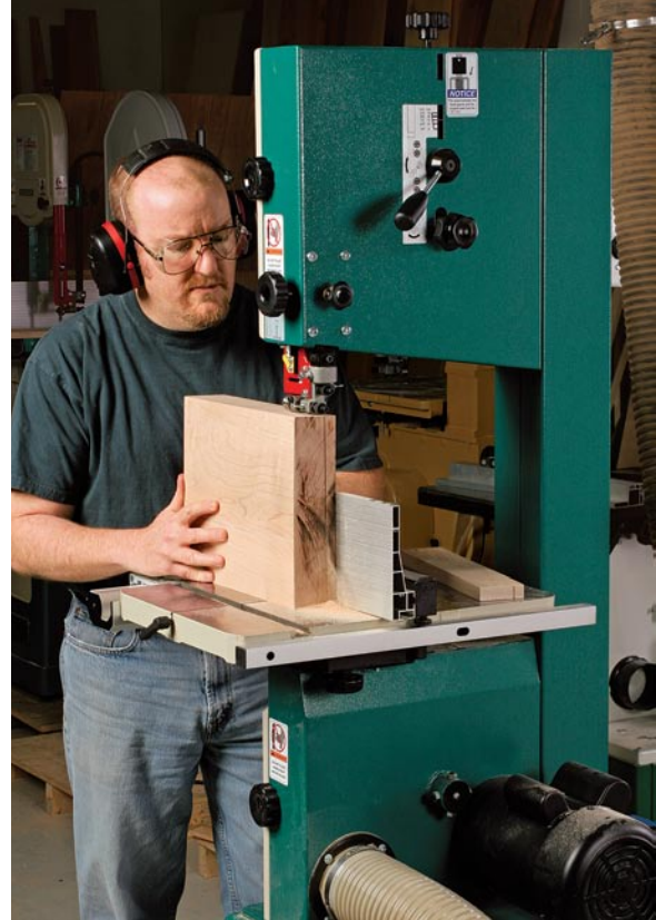
Resaw beast. The Grizzly 14-in. bandsaw comes with a tall fence and plenty of muscle to resaw wide stock.
