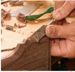
How to control it. Using the bevel of the chisel in the same way as the sole of a spokeshave allows you to get into tight spaces, such as the beveled edges of this chair splat, with perfect control.
