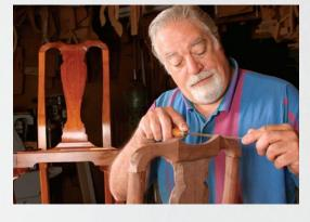
can do the job, the hand tools are often quicker to use, especially if only one or two pieces of wood are involved. A power tool may require considerable setup time, whereas you can just whip out these hand tools and start making shavings.
