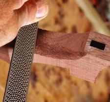
Fast cutting. A coarse rasp removes wood quickly, especially when used at 90° to the grain. To avoid creating deep grooves, look for a rasp with teeth that are not in a straight line, lengthwise.
