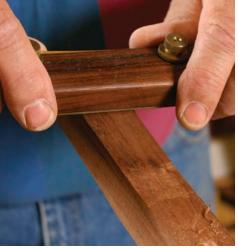
**Tight mouth, thin shavings.** After creating the basic profile with a metal spokeshave, Sharp uses a wooden shave with its low blade angle and tight mouth to work areas of tearout.
