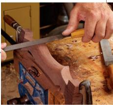
File a smooth surface. A coarse/ medium file cleans up any remaining rasp marks and leaves the surface ready for scraping and sanding.
