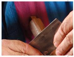
**Scrape long curves.** A scraper quickly removes the facets left by the spokeshave, fairing the surface into a smooth curve.
