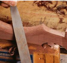
Less aggressive. A medium rasp removes the lines left by the previous rasp. Tapered, half-round rasps are the most useful for shaping wood.
