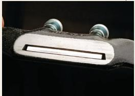
Close the throat. Make a dense hardwood shim (left) that fits between the frog and blade. The shim shouldn't be so thick that the blade no longer engages the adjustment screws. The tighter throat (right) makes for much smoother
