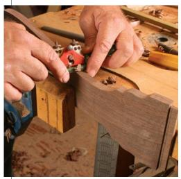
**Smooth curves.** A flat-bottomed spokeshave can work a concave surface down to about 10 in. dia. To go with the grain, work downhill from both directions.
