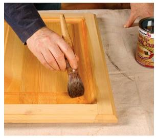
**Lock it in.** Before topcoating, seal the surface with a couple of coats of dewaxed shellac.
