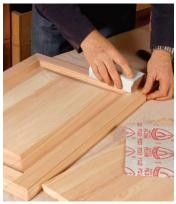
Raise the grain. Wipe the whole surface with a wet cloth and let the wood dry for two to four hours. After the wood has dried, the surface will feel rough. Lightly sand it with P220-grit paper and remove the dust. The surface can now receive the water-based dye without swelling up.
