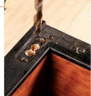
**Mark and mortise.** With the hinge in place, mark the location of the stay mortise. Remove most of the waste with a drill, then square up the sides with a chisel.
