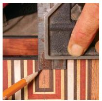
**Locate the key pin.** Measure the distance from the top of the lock to the key pin and mark the location.
