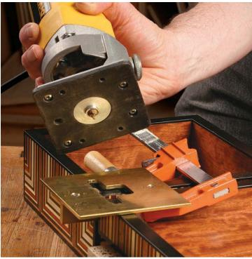
**No chisel work.** Although you can cut the hinge mortises by hand, it is much quicker and more accurate to use a dedicated router template in conjunction with a straight bit and a bushing guide.
