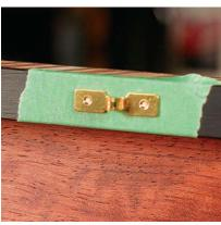
**Stuck in the right place.** Place some green tape on the lid and close it, pushing down onto the lock. Reopen it with the double-faced tape holding the catch in perfect position.
