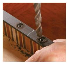
Define the shallow mortise. Use a larger brad-point or Forstner bit to drill partway into the screw holes. This will create the two ends of the mortise for the lock's selvedge. Now you can scribe the edges of this shallow mortise and chop out the rest with a chisel.
