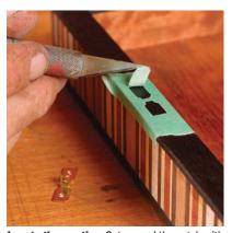
**Locate the mortise.** Cut around the catch with a sharp knife, severing the green tape. Remove the catch, peel away the cut tape, and mortise these areas.
