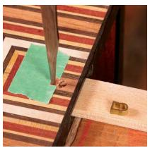
**Cut the keyhole.** After drilling a hole to locate the key pin, remove the lock, insert a scrap of wood to fill the lock mortise, and chisel a hole for the key and the escutcheon.
