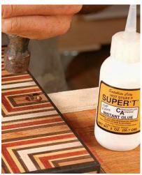
**Install the escutcheon.** Use a mixture of cyanoacrylate glue and sawdust to attach the escutcheon. File and sand it flush with the wood.
