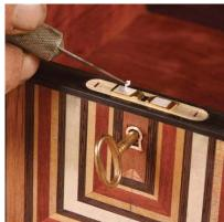
Use double-faced tape. With the catch locked into the body of the lock, apply two small pieces of double-faced tape to the back of the catch.
