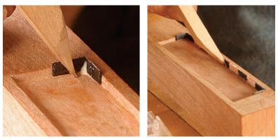
**Start in the corners and work your way toward the middle.** Hack uses the tapered end of a stick to push the bottom of each segment into place (above). Then he uses the square end of the stick to press them against the wall of the recess (right).
