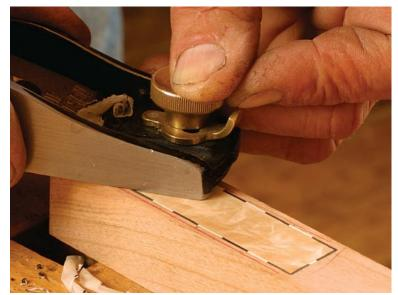
The last step. When the glue is completely dry, bring the panel and border flush, skewing the plane to avoid tearout on any of the pieces, which are running in various directions. A scraper might be helpful for the last few passes.
