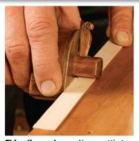
**Thin slices, please.** Use a cutting gauge or a marking gauge to slice <sup>3</sup>/<sub>16</sub>-in.-wide strips of the border material. The strips will break away with ease along the kerf.
