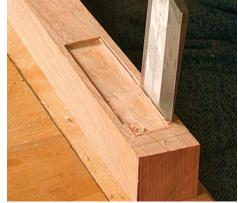
**Use chisels for the fine work.** Chop up to the knifed lines with chisels. Be sure to keep the walls of the recess vertical as you chop; otherwise, you may have trouble fitting the parts.
