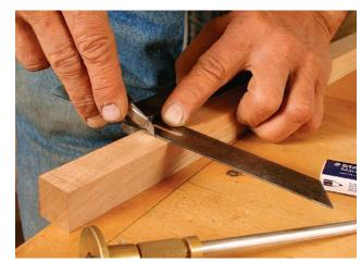
**Knife in the outline.** The knifed lines will help prevent tearout at the top of the recess and will serve as a guide for the chisel work. Use a cutting or marking gauge for the long sides (left), and a knife and square or bevel gauge for the ends (above).
