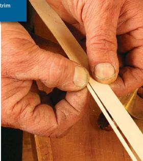
**Clean up with a block plane.** Hack planes the stock on a flat scrap board, with a hardwood dowel as a stop. Plane the strips to <sup>1</sup>/16 in. thick, being sure to keep them all the same thickness so the border will have a uniform appearance.
