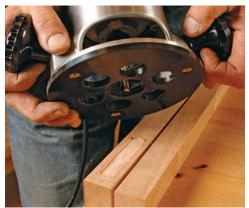
**Rout to the red.** Use a <sup>3</sup>/<sub>16</sub>-in. straight bit, set to a depth just under the panel's thickness, and stay within the red lines. Use a spare leg to help support the router base.
