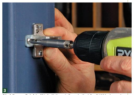
**Attach the mounting plate.** Align it with the centerline and setback line. Hold it in place, and drill pilot holes. Then drive in the mounting screws. O'Malley is using a self-centering bit here.
