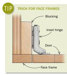
Cup hinges designed specifically for face frames are clunky and unattractive. They are also screwed to the edge of the face frame, which can cause the wood to split. Use one designed for a normal inset door on a frameless cabinet instead. Install some blocking behind the frame for the mounting plate, and then installation and adjustment are the same.
