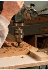
**Bore a hole for the hinge cup.**Mark the hinge centerlines on the door. Then use a 35 mm Forstner bit to drill the mortises.
