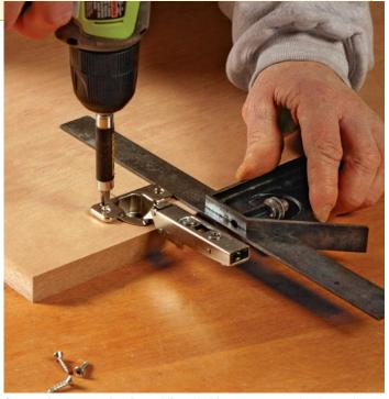
**Screw the cup to the door.** Align the hinge square to the door edge with a combination square. Then screw it to the door.
