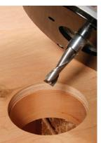
**ROUT THE HOLE WITH A SINGLE PASS**
