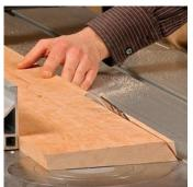
**Edges last.** Leave the blade at 60° and bevel the outside edge of the seat slat.
