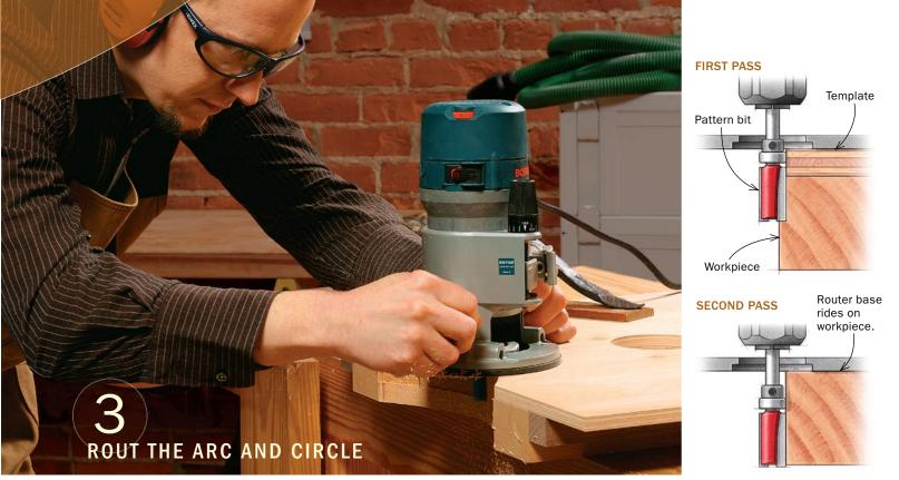
**Rout the arc.** Because the legs are 1¾ in. thick, it takes two passes with a pattern bit to rout the arc flush. On the first pass, the bearing rides against the template. For the second pass, remove the template and register the bearing against the routed surface (see drawings above).
