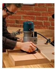
**Groove the glueline.** Use a ¼-in. straight bit to rout a ¼-in.-deep groove over the glueline.
