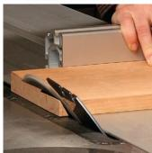
Ends get a compound angle. With the blade tilted to 60° and the miter gauge set at 89°, crosscut the slat to length. The outside edge should be against the fence. For the second cut, move the miter gauge to the other side of the table and turn the board over.
