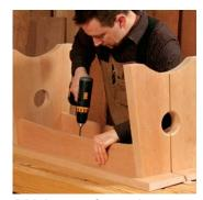
Add the seat. Secure the top with pocket-hole screws. Note the ¼-in.-thick spacer on the bench keeping the tapered slats flat against the legs.
