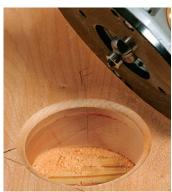
Cove the edge. A ¼-in. bearingguided cove bit routs a nice detail on the outside edge of the hole.
