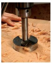
walls of the hole. The template allows you to drill the hole undersize and rout it to finished diameter with a spiral bit, leaving a smooth surface.
