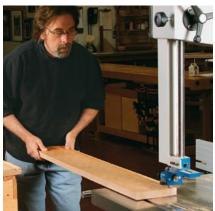
**Bandsawing is safer.** Ripping the unjointed boards on the tablesaw might cause kickback. So cut them ¾ in. over final width on the bandsaw.
