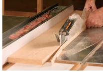
**Joint one edge, then rip to width.** Run one edge over the jointer until it is flat and at 90° to the face that is against the fence (left). With the jointed edge against the fence of the tablesaw (right), rip each board slightly over final width.
