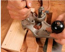
**Define and relieve.** A shopmade scratch stock marks the inside edge of the bead and establishes the fillet (top). Breed uses a router plane to relieve and flatten the area from the scratch line toward the center of the table (bottom; note the spacer blocks on the bench and in the center of the table that stabilize the plane), further defining the bead and fillet.
