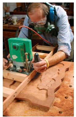
**Establish the flat field.** To create the look of an applied molding, the material in the center of the top has to be subtracted. Breed uses a 2-in. Forstner bit to waste away most of the recess. To remove the rest, he switches to a router attached to a frame. The frame rides on the outside edges of the table while he guides the router freehand close to the line. Chisels and gouges take the shape to the line.
