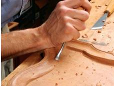
**Shape in two steps.** After establishing the sharp corners in the miters with a V-tool, Breed uses a 7/20 gouge to create the hollow in the molding (top). A backbent gouge is used to round the bottom of the ogee profile (bottom). To smooth the carving, Breed uses two customized scrapers ground to match the hollow and round of the ogee profile.
