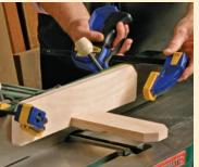
Changing of the guard. The typical blade guard won't let you surface a board that's wider than the jointer tables, so you'll need to replace the stock guard with a shopmade version.
