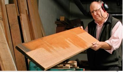
**More work required?** A board with extra cup, bow, or twist won't be flat enough after one pass. If the infeed table is no wider than the knives, just make extra passes. Otherwise, you'll need to make a simple auxiliary table.
