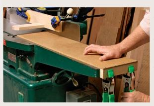
No tipping allowed. The auxiliary table acts as a shim, preventing the board from tipping as you make additional passes. Clamp the stop block to the infeed table to keep it from shifting.
