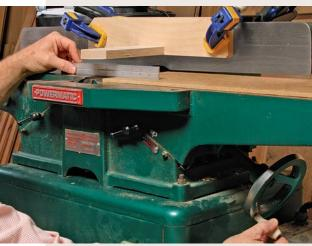
**Set the table.** Lower the infeed table until the surface of the auxiliary table is flush with the outfeed table; then lower the infeed table a bit farther to produce a light planing cut.
