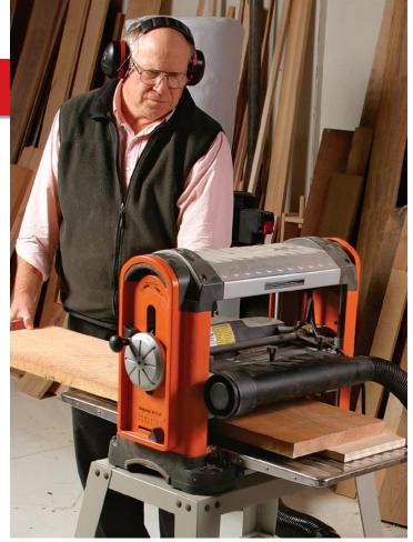
**Plane the top surface.** With the plywood spacer face down on the planer bed, make light passes as needed to flatten the opposite surface of the board.
