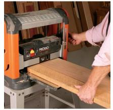
**Now the other side.** After the top is flattened, remove the spacer from the rabbet. With the flattened face of the board on the table, lower the cutterhead (above) so the thickness planer will make a light planing cut on the step. Make passes until the step is gone and the whole surface is smooth (right).
