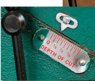
Cut a shallow rabbet. With the jointer fence set to make the widest possible cut and the infeed table set to make a cut 1/16 in. to 1/8 in. deep, feed the board across the cutterhead to make a wide, shallow rabbet (right). If the board is reasonably flat from the get-go, a single pass on the jointer produces a rabbet that's perfectly flat and straight (below). See p. 70 if additional passes are needed.
