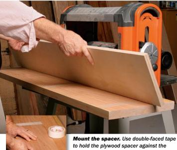
**Mount the spacer.** Use double-faced tape to hold the plywood spacer against the rabbet. Press the parts together to make sure the tape sticks.
