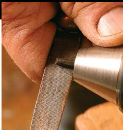
Dots are easy to make. Chuck a narrow blank of ebony into a drill and use a file to shape the blank into a 1/8-in.-dia. rod (left). Slice off a 1/8-in.-thick section and glue it into the tip of the fan (right).
