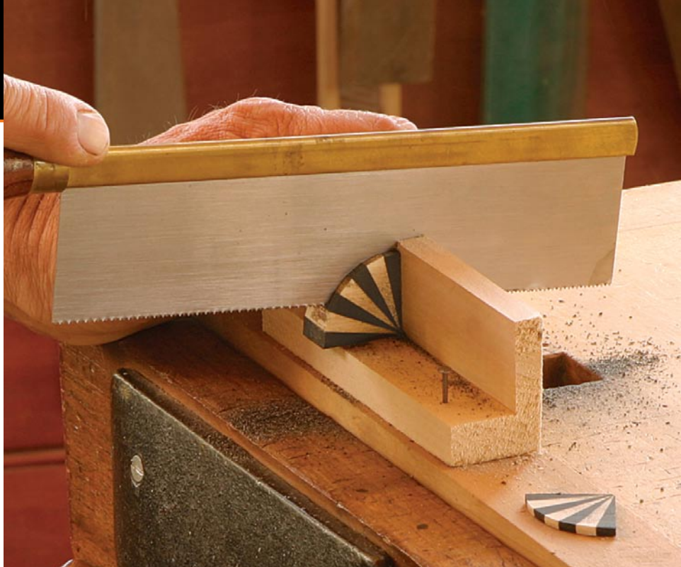
Thin slices, please. Use a dovetail saw to cut the ⅛-in.-thick slices. An L-shaped block, tacked to a scrap clamped in a vise, acts as a bench hook to hold the small pieces.
