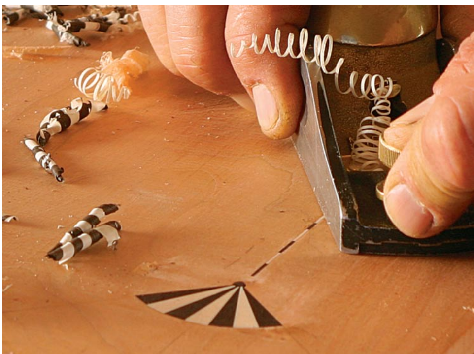
Plane everything smooth. Use a block plane to level the inlay, then work the entire surface with a smoothing plane and/or scraper.
