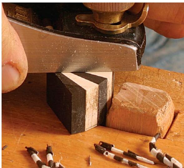
Get rid of the crust. Clean up the sandwich faces using a block plane.
