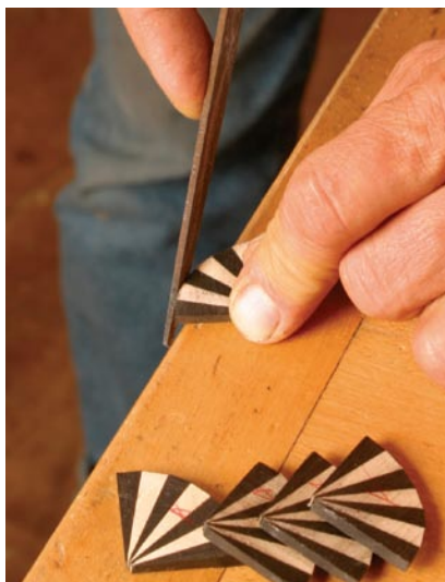
Smooth the outside and make a home for the dot. Fair the curved surface using a file (left) or sandpaper, then use a ⅛-in.-dia. file to form a shallow recess in the point of the fan (right).
