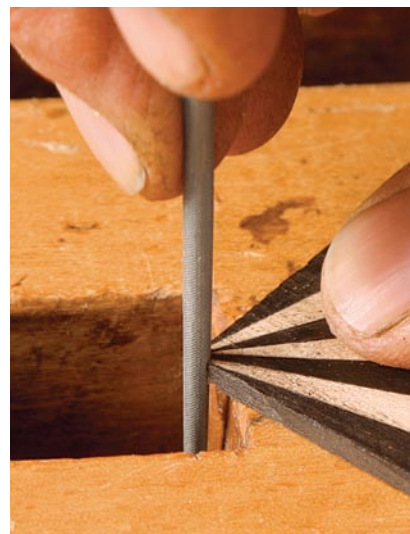
Smooth the outside and make a home for the dot. Fair the curved surface using a file (left) or sandpaper, then use a ⅛-in.-dia. file to form a shallow recess in the point of the fan (right).
