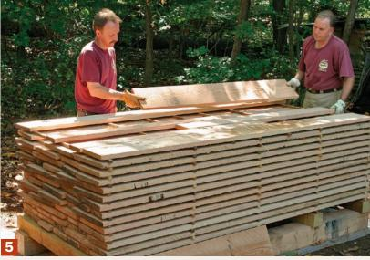
Short boards are OK. When encountering an odd length, such as a 5-ft.-long board that doesn't divide into 2-ft. intervals (or 18-in. intervals for softwood), add an extra sticker to the layer so both ends are supported.
