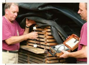
**Check back often.** Every couple of months, measure your drying progress using a moisture meter. Pick a board in the middle of the stack.
