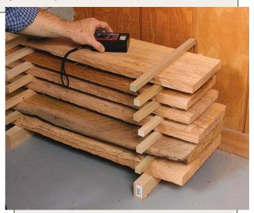
**Stack and sticker indoors, too.** Use stickers to ensure good airflow between boards. Check the MC every couple of weeks with a moisture meter until they get to their target moisture content.
