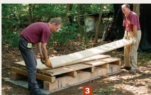
Start stacking. Use the lowestquality boards for the bottom layer (3). When wide boards go near the bottom, the weight of the other boards above helps keep them flat. Also, the stack will be more stable if the gaps between boards are staggered from layer to layer (4).
