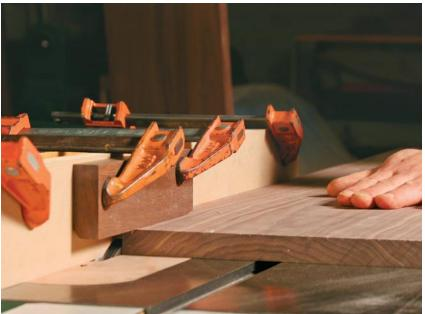
**Bury the cutterhead.** Turn on the saw and raise the cutter. Creep up on the right height by taking test cuts. Then adjust the fence for the right rabbet width. When cutting rabbets, clamp a block over the cutterhead. The block will hold down the workpiece, so you can keep your hands away from the blades.
