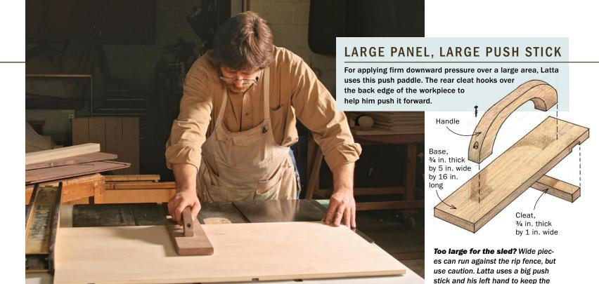
from the fence, creating a kickback danger. Again, depending on your saw's design, a stub splitter in this setup can radically reduce the chances of this happening.
