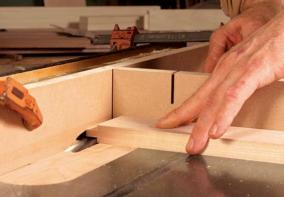
**Cut the stub tenons with a rabbeting setup.** Use a miter gauge with an auxiliary fence to bring the work to the cutter. This is one time you can use the miter gauge and rip fence at the same time.
