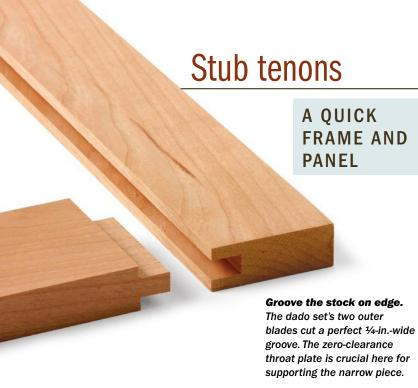
this assembly works well for lightweight doors, dust panels, and other light-duty applications. With a plywood panel glued in, the assembly will be strong enough for the most demanding situations.
