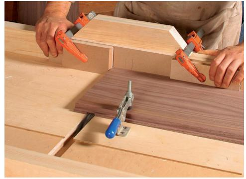
**Two extra touches.** A stop block ensures matching workpieces. A toggle clamp screwed to the deck of the sled and a block clamped to the fence help hold down long stock like this case side.
