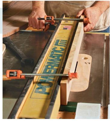
blades wider than the rabbet you plan to cut. If you're running a 3%-in. rabbet, for instance, mount a 1/2-in. stack and bury at least 1/4 in. of it into the MDF to create the opening in the sacrificial fence.
