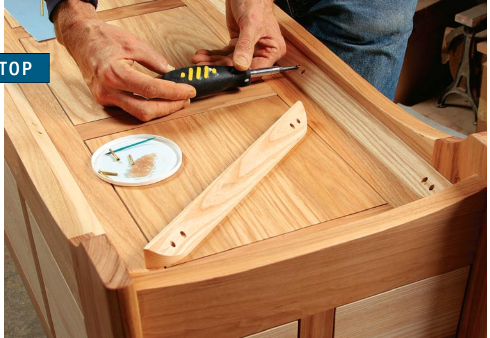
Fit and secure the bottom. The ledger strips have pairs of holes: One is for screwing the strip into the side of the chest (above), and the other is for fixing the bottom in place.
