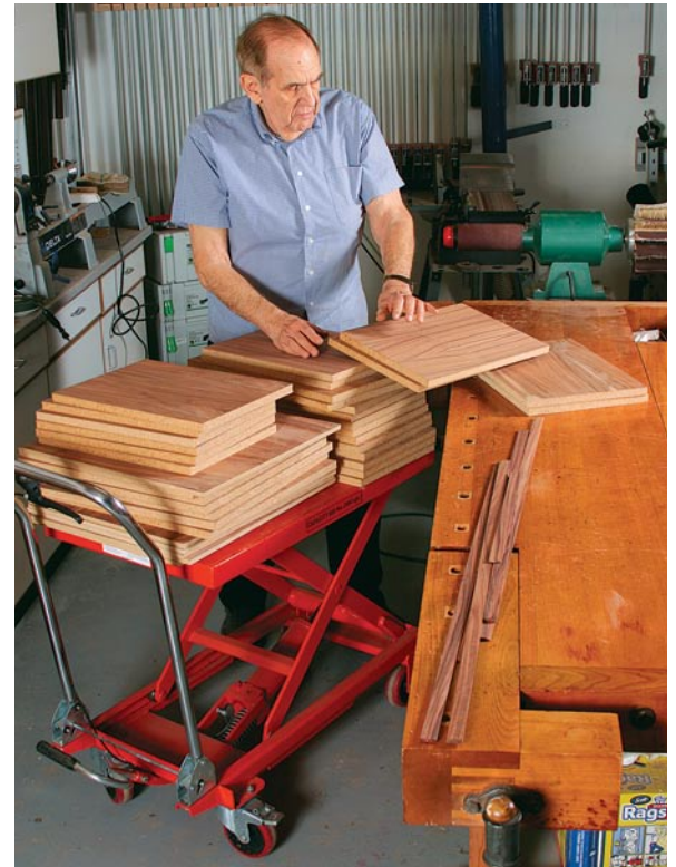
A little pick-me-up. A scissor-lift cart lifts heavy materials to bench height, and makes a multilevel work surface.
