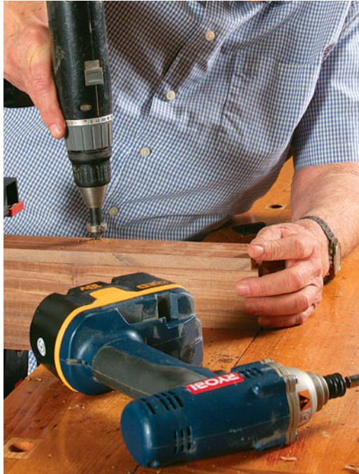
One for drilling, one for driving. The combination of a cordless drill and an impact driver can save you lots of grief.
