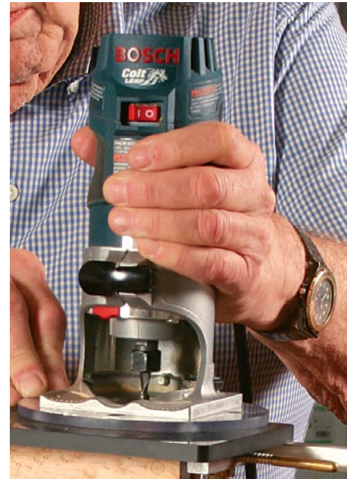
One-handed routing. For light-duty tasks such as mortising for a hinge, a lightweight router is much easier on hands and wrists.
