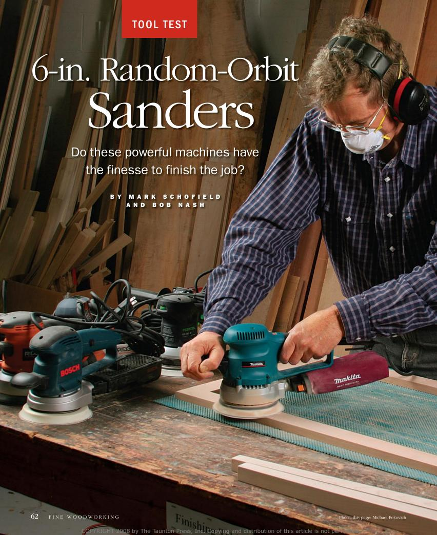
ne inch doesn't seem like much, but when it comes to randomorbit sanders, it makes a large difference. For starters, the pad on a 5-in.dia. sander is 19.6 sq. in., while that on a 6-in.-dia. model is 28.3 sq. in., giving you 44% more sanding surface. To drive this extra capacity, 6-in. sanders have more powerful motors, and many work in two modes—coarse and fine. The smaller sanders operate only in fine mode.
