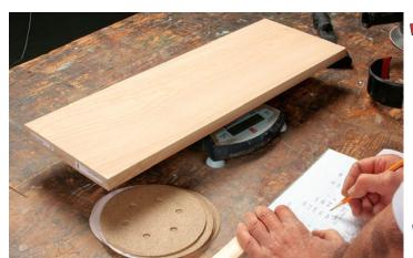
Stock removal. Using scales accurate to 1 gram, a cherry board was weighed before and after each five-minute sanding test to calculate the amount of wood removed (above). To see how much dust was collected by the vacuum, it was weighed before and after each test (right).
