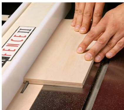
Grooves for the bottoms. Run the bottom of the sides, fronts, and backs against the fence to cut the groove for the bottom panel.
