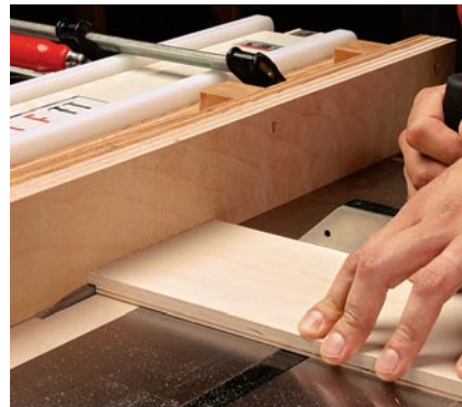
Rabbet the fronts and backs. With the dado head buried in a sacrificial fence, cut the rabbets for the corner joints.
