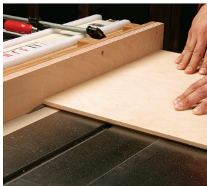
Rabbet the bottom panels. All four sides of the bottom panels are rabbeted to fit into the grooves running around the bottom of the drawer box.
