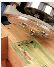
Slots are added after construction. A router template (shopmade or store-bought) can be clamped to the workpiece (above). A plunge router equipped with a guide bushing and keyhole bit rides in the template to cut the slot (left).
