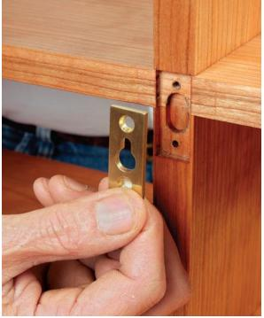
Cut a mortise for the hardware. After scribing around the hanger, freehand rout to a level that equals its thickness, and then use a chisel to clean to the line. Then rout a deeper slot to accept the screw head. Make sure to leave enough wood on the first level to secure the hanger with screws. Mortising the hardware allows the work to hang flat against the wall.
