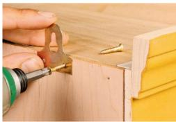
Above eye level. The ideal situation for rigid hangers is a cabinet like this one. The crown molding is above head height and also extends beyond the top of the case, concealing the hangers.
