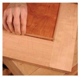
Fit it piece by piece. Glue the molding to the frame only, not to the panel. Work on one piece at a time, marking, cutting miters, and gluing as you go. Use hand pressure to keep the pieces in place for about 1 minute each, and then leave a few pieces of tape behind as clamps.
