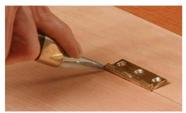
**Transfer the location to the carcase.** Once the hinges are screwed to the doors, position them in the opening, leaving the gap you want along the top and bottom edges. Use a marking knife to transfer the hinge placement, and then remove the door (and unscrew the hinges), set the hinges in place on the edge of the frame, and mark around them.
