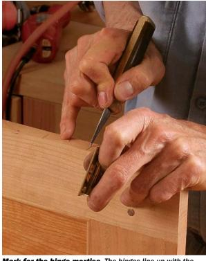
Mark for the hinge mortise. The hinges line up with the top and bottom rails. Hold the hinge in place and trace around it lightly with a knife. Then remove the hinge and cut heavier lines to rout to and place the chisel in later.
