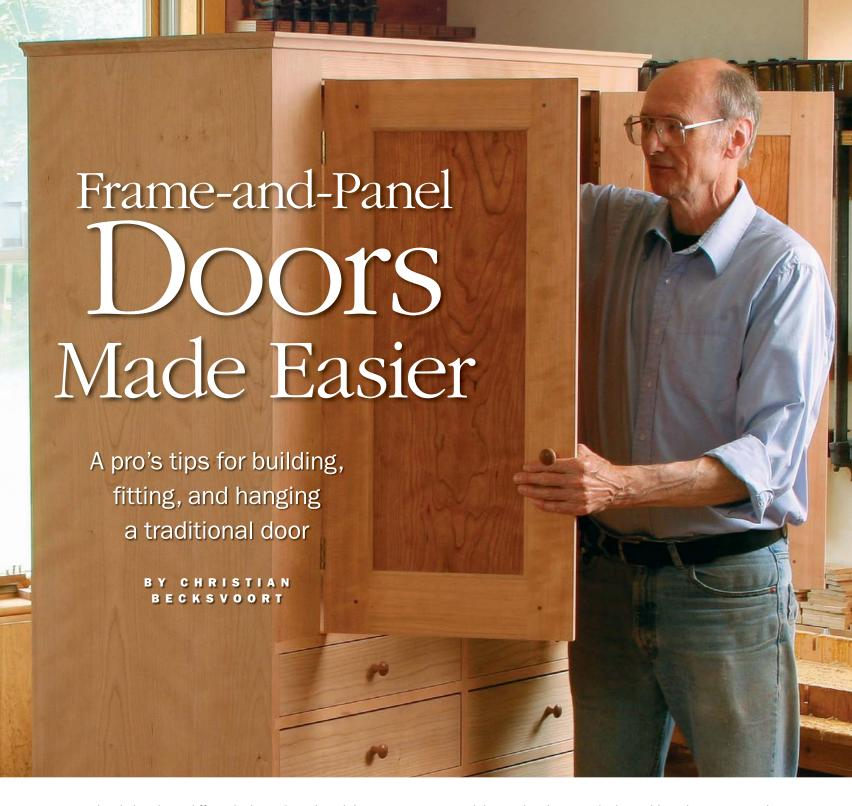
make Shaker doors differently than others do. While you can't beat a mortised-and-tenoned, pegged frame for strength and style, I prefer a thin, inset panel surrounded by a quarter-round molding as opposed to raised-panel or pillowed-panel doors. Although the Shakers used moldings sparingly, the quarter-round along the inner edges of the frame makes for a clean, slightly rounded, and understated design. This style can blend into both period and modern environments.
