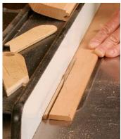
**Cut the molding.** A wide work-piece is easier and safer to machine. Cut the quarter-round profile on the router table (profile both sides of the piece), and then rip the moldings to width on the tablesaw.
