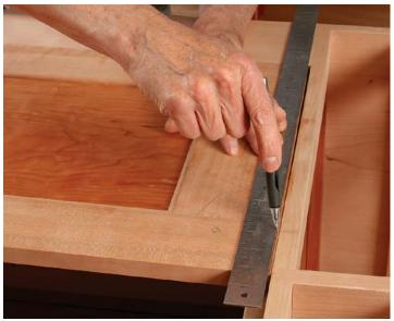
Fit the length first. If the door isn't parallel to the case, you'll have to make an angled cut. Working on one door at a time, butt the door to the hinge side and mark the door parallel to the bottom of the opening.
