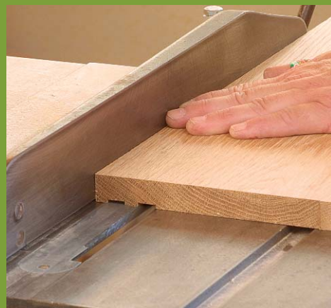
Cut grooves for the lower track. These shallow grooves can be cut directly into the cabinet bottom.
