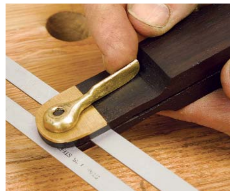
Locking lever. The Gladstone tool uses a lever that sits below the side of the body and is easy to use.
