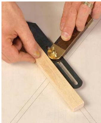
Get an angle from a drawing. A block of wood aids in taking an angle directly from a drawing.
