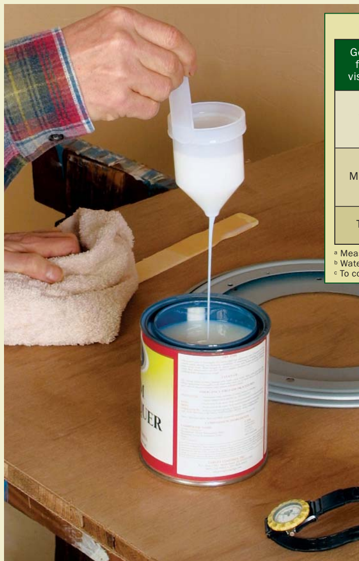
Measure the viscosity. Submerge the viscosity cup in the finish and time how long it takes for the stream of finish to break.
