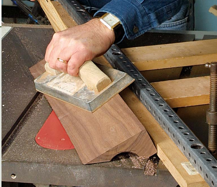
Apply steady pressure and take small bites. Because the workpiece is being pushed across the blade and not through it, the blade should be raised by only \frac{1}{8} in. for each pass. Push down and toward the fence with a large padded push block, such as this tile-grout trowel, and forward with a push stick.
