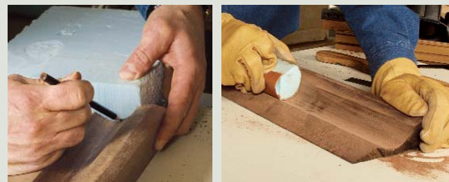
Shopmade profile sander. Transfer the shape of the cove onto some building foam (left) and then cut the foam to shape on a bandsaw. With sandpaper wrapped around the custom-shaped foam block (right), sanding the cove goes smoothly.
