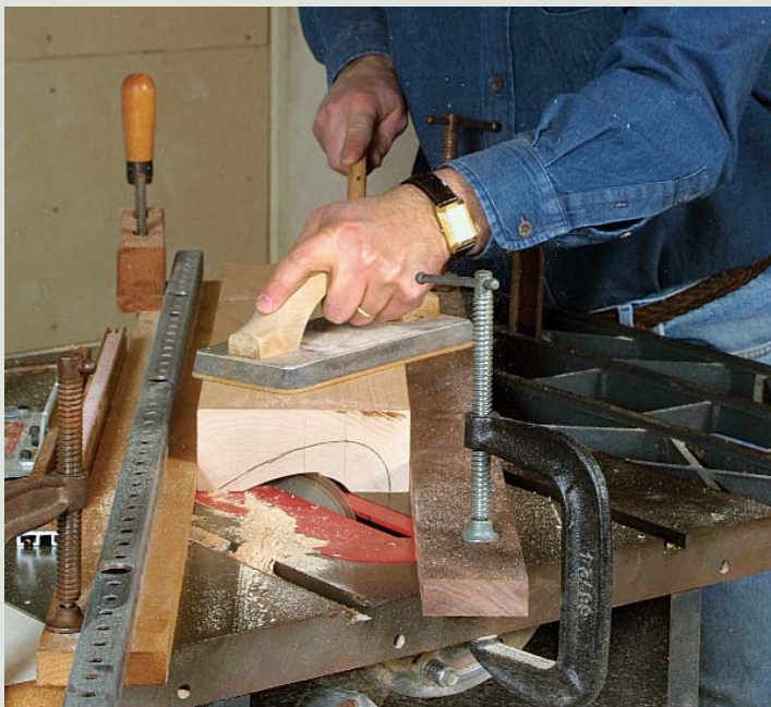
Feed into the tilting blade. The workpiece should approach from the side that the blade is tilting toward. Otherwise, there is a risk that the workpiece may slide up the sloping blade and over the front fence.
