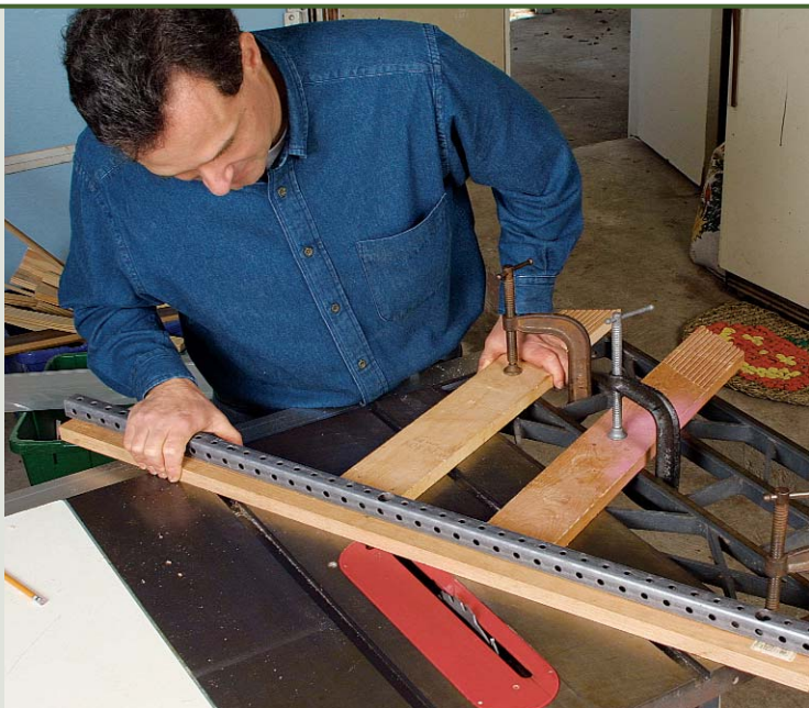
Clamp the fence. Once the fence angle and the offset distance have been set, clamp the fence securely to the table. If it is difficult to set a clamp on the front rail, use braces clamped to the extension table.
