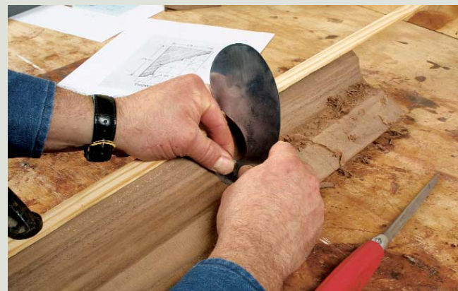
Scrape away sawmarks. A gooseneck scraper should fit any cove profile. Turn an edge on the scraper with the burnisher.
