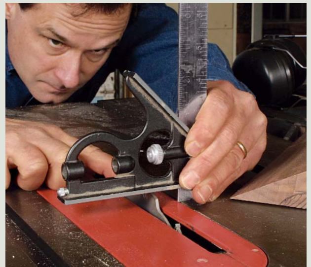
Setting the blade height for a symmetrical cove. Raise the blade to match the depth of the cove. The blade is lowered after the setup to cut in \frac{1}{8} -in. increments.
