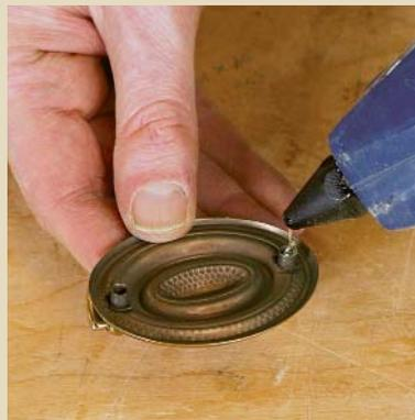
**Experiment with the location of hardware.** To avoid damaging the drawer front, apply only a tiny bead of hot-melt glue to the back of the pull (above) and press it in place (right).
