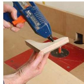
**Handling small pieces safely.** When pattern-routing a small piece, it is safer to attach it temporarily to a larger piece of wood using hot-melt glue.
