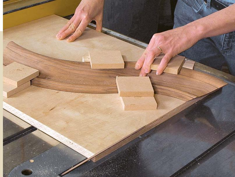
**Well secured.** Blocks on both sides of the gooseneck molding lock the workpiece to the plywood carrier. Secured to the carrier, the gooseneck miter can be trimmed using the rip fence as a guide.
