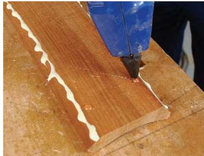
First apply yellow glue to the molding for the permanent bond. Add a few small blobs of hot-melt glue just inside the yellow glue (above). Locate the molding quickly before the hot-melt glue hardens (right). The hot-melt glue holds the molding in place while the yellow glue sets.
