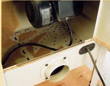
An access door and a perforated tray. The Jet SuperSaw has a fairly airtight base, accessed through a hinged door. Johnson thinks the tray with holes in it on the Jet SuperSaw will work well with fine sawdust, but he found that some dadoing and ripping operations will cause it to clog up.
