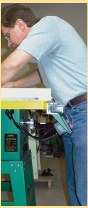
This switch gets in the way. Switches on the Bridgewood and Woodtek saws project past the plane of the front rail of the fence, so they're easy to bump into.
