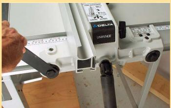
The Delta Unifence is unique. To adjust the Unifence square to the sawblade, you use the same wrench supplied with the saw for changing blades. The extruded-aluminum fence can be located in either a high or a low profile, to adjust for different ripping operations. Extruded flanges wrap around a flat metal bar that holds the fence tightly to either side of the main carriage to which it's attached.
