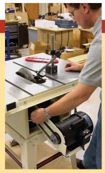
saws use machined iron pulleys. A few of the saws could benefit from higher-quality belts, but most of them ran smoothly with little or no vibration. Only the Grizzly comes equipped with a link belt, which reduces vibration and makes the saw run more quietly.
