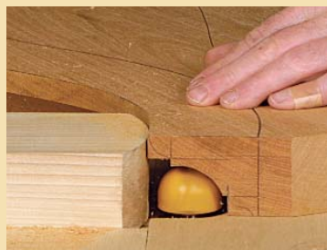
Next, cut the cove. Take multiple passes using a large half-round (core-box) bit.
