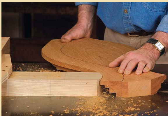
Start with a large 8/4 slab. Bandsaw the lower edges of both moldings from one slab, which provides a stable platform during routing.
