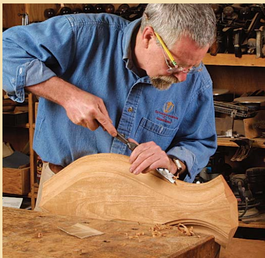
Next, cut the cove. Take multiple passes using a large half-round (core-box) bit.
