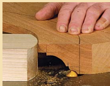
Cut the cyma recta. Start with a 1/4-in.-radius roundover bit. Finish with a 3/4-in. half-round (core-box) bit.
