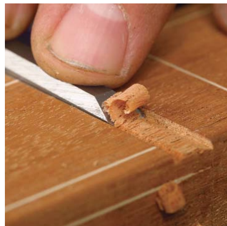
Chisel away the waste. Start with ramp cuts with a wide chisel (left). Then switch to a narrow chisel to clean the bottom of the dado (right).
