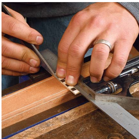
Scribe the edges of the dado. Carry across the upper line from the apron. Then use a piece of banding to locate the lower edge.
