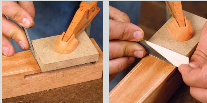
Scribe the rectangle. After penciling in the layout, use the scratch stock to cut the vertical grooves. Then use a block as shown (left) to scribe one side of the top and bottom grooves. Next, use a piece of the stringing veneer as a guide (right) to scribe the other side of each groove.
