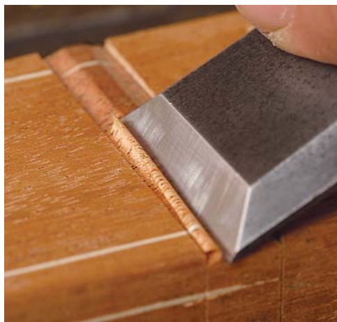
Chisel away the waste. Start with ramp cuts with a wide chisel (left). Then switch to a narrow chisel to clean the bottom of the dado (right).
