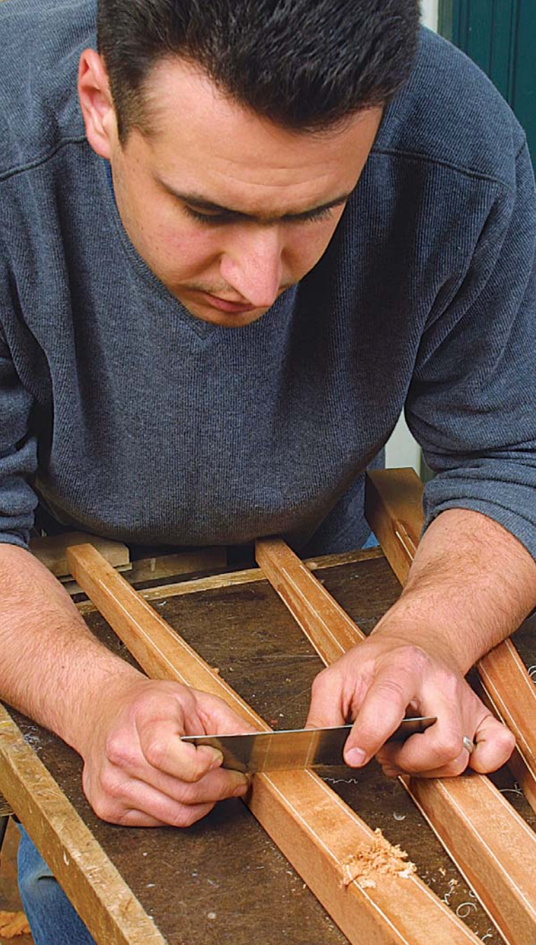
Last, scrape the surface flush. Scrape just enough to clean the surface but not enough to cut beneath the shallow stringing.
