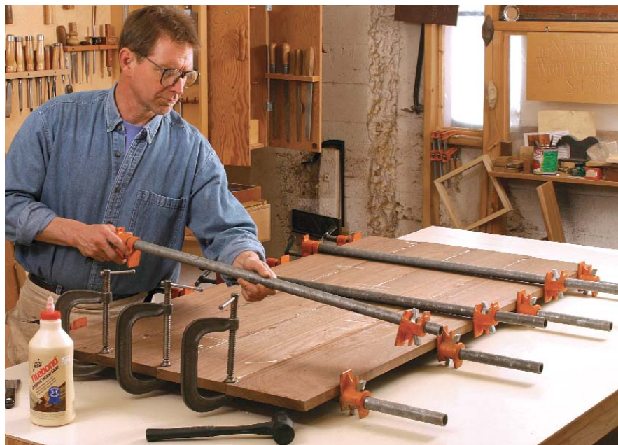
Add the top clamps. Placing clamps on top helps balance the clamping forces applied by the bottom clamps. If all of the clamps were mounted on only one side, the panel likely would buckle when the clamps were tightened.
