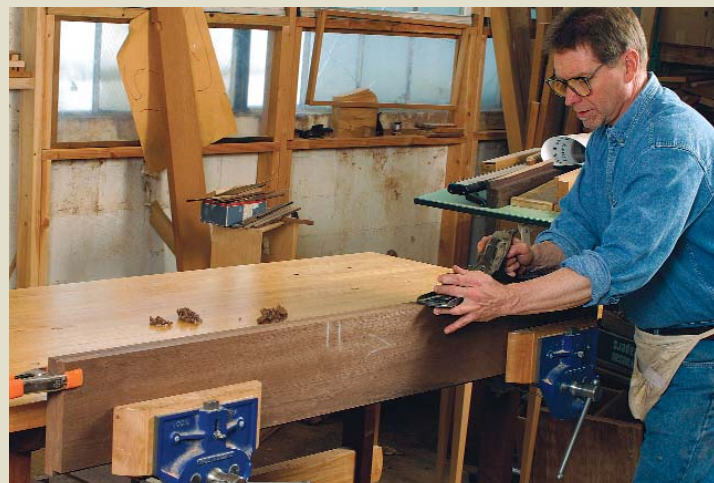
No jointer? No problem when you plane in pairs. The joints can be handplaned with the mating edges of the boards held flush in a vise.
