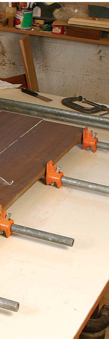
C-clamps keep joints flush. With the pads of a C-clamp temporarily spanning the joint lines at each end of the boards, the faces of the boards won't slide out of alignment.
