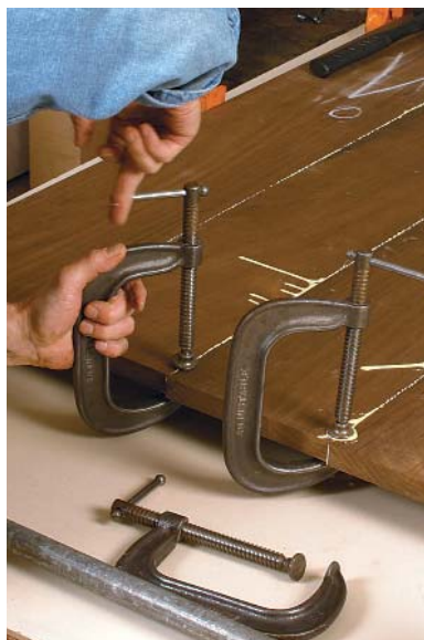
C-clamps keep joints flush. With the pads of a C-clamp temporarily spanning the joint lines at each end of the boards, the faces of the boards won't slide out of alignment.
