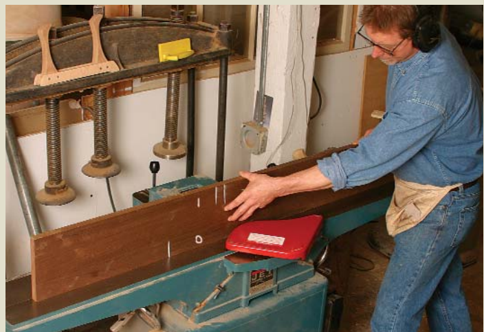
Jointing the edges. When using the jointer, pay attention to the face-orientation marks.
