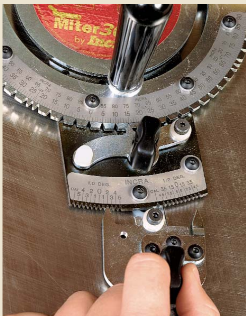
Setting angles is less straightforward on the 3000. The big rack has stops every 5°, and the smaller rack is used to add single and half degrees to those settings.
