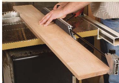
The longest crosscut capacity. The telescoping arms and extension block allow the stop on the EB-3 to work on boards as long as 42 in.
