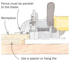
Use a spacer or hang the workpiece off the edge of the bench to ensure that the base is not resting on the benchtop.
