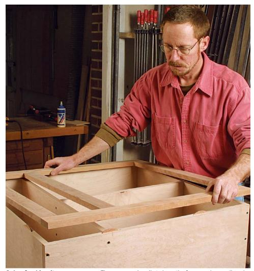
**Only a few biscuits are necessary.** These serve primarily to keep the frame and case aligned during glue-up. Use plenty of clamps to distribute pressure. The glue-up will go more easily if the piece is on its back with room all around for clamps.
