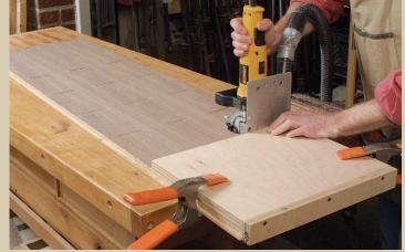
**A jig to locate multiple fixed shelves.** For a symmetrical series of shelves, use a piece of sheet stock that reaches to the center shelf. A small cleat at the end locates the jig accurately each time (right).
