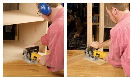
**Use the tool's base as the reference.** Cut the slots in the case as usual, but place a ¼-in.-thick shim under the tool when slotting the face-frame stiles.
