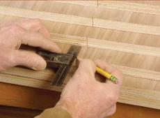
**Layout tricks.** For this carcase, only the center of three biscuits must be marked. To locate the outside biscuits, line up the edge of the tool with the edge of the stock. Mark the pieces as a group, first on their ends (left), carrying the marks onto the faces where necessary (right).
