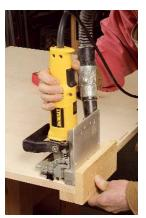
The standard position is shown at left. To cut the mating slots, the workpieces or the tool (above, with the help of a jig) must be positioned vertically.
