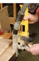
Fence adds convenience. If the fence is used for both cuts (left and above), the workpieces can remain flat without the need for jigs.
