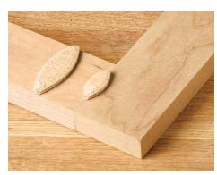
**Narrow frame pieces require smaller, nonstandard biscuits.** The Porter-Cable 55K Plate Joiner includes a smaller blade for joining pieces as narrow as 1½ in.
