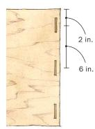
A good rule of thumb for carcase construction is to 2 in. use at least one biscuit for every 6 in. of width. Locate them close to the front and back edges to keep the corners aligned, unless screws are used for assembly.
