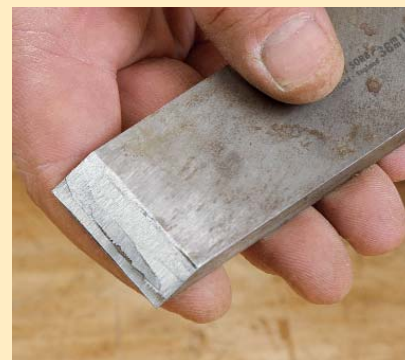
Getting there. With rust and dried glue ground away, this bevel is ready for abrading on the stone.
