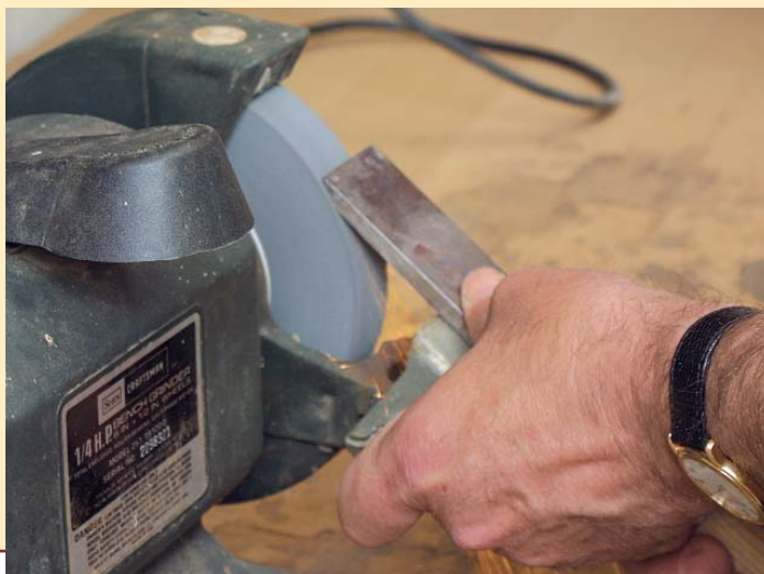
Clean up the bevel first. With new aluminum-oxide wheels (60/80 grit and 100/120 grit) installed on an old grinder (above), Duckworth removes the crud from the bevel (right). Aluminum-oxide wheels are better for grinding woodworking tools because they don't overheat and ruin the steel, which can happen easily with silicon-carbide wheels.
