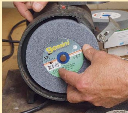
Clean up the bevel first. With new aluminum-oxide wheels (60/80 grit and 100/120 grit) installed on an old grinder (above), Duckworth removes the crud from the bevel (right). Aluminum-oxide wheels are better for grinding woodworking tools because they don't overheat and ruin the steel, which can happen easily with silicon-carbide wheels.
