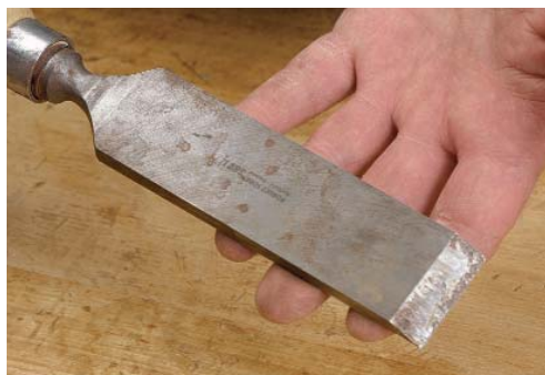
Before. This mortise chisel, covered with glue globs and rust and as dull as a butter knife, has seen better days.
