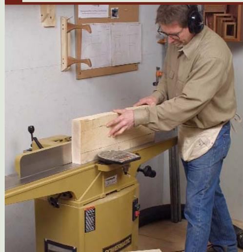
**Joint one edge.** It's not important that the edge be square to a face; it just has to be straight and flat. Check grain orientation to get a smooth cut.
