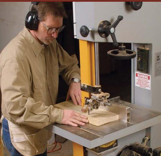
**Rip to  $\frac{1}{8}$  in. over in width.** The bandsaw is a safer tool for ripping rough lumber than the tablesaw, which is prone to kickback. The bandsaw also wastes less material.
