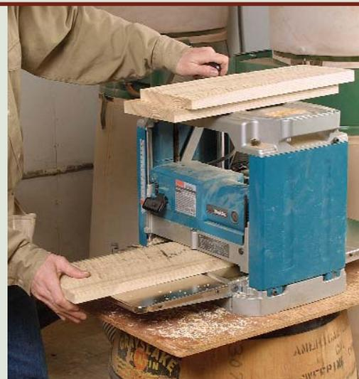
**With the jointed side facedown, run the boards through the planer.** Once both faces are flat, alternate faces to take off similar amounts from each side until the finished dimension is reached.
