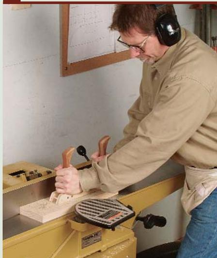
**Joint the first face.** Start the finish-milling process by jointing one face flat. Use push sticks or pads to hold down the stock, concentrating pressure just past the cutterhead.
