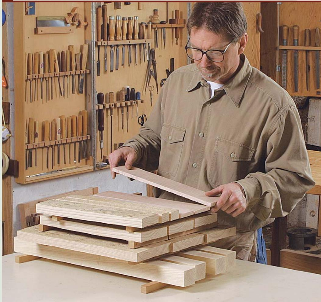
**Stack it and wait.** Layer parts between stickers to let air circulate. Allow a week or more for the parts to move slightly and stabilize.
