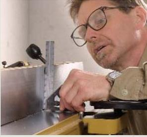
**Edges are next.** First, check the jointer fence for squareness (above). Check just past the cutterhead. Joint one edge square, flat, and straight (right), using push sticks or pads when your fingers would pass near the cutterhead.
