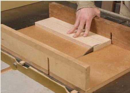
**Ends are last.** Use a tablesaw sled to cut the ends accurately. Square up one end first (above), then clamp a stop on the sled to cut the other end (right).
