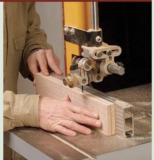
**Mill to rough thickness, if necessary.** If the stock must come down more than  $\frac{1}{4}$  in. in thickness, flatten one face on the jointer (left), then resaw or plane to  $\frac{1}{8}$  in. over in thickness (right).
