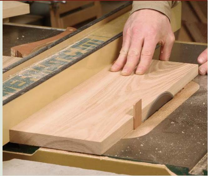
**Mill the final edge on the table saw.** Note that this is the first time the table saw has been used during the milling process, and only to remove a small amount of wood.
