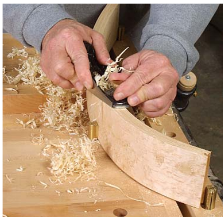
One edge is handplaned. When removed from the form, the edges of the workpiece are uneven and covered with glue.
