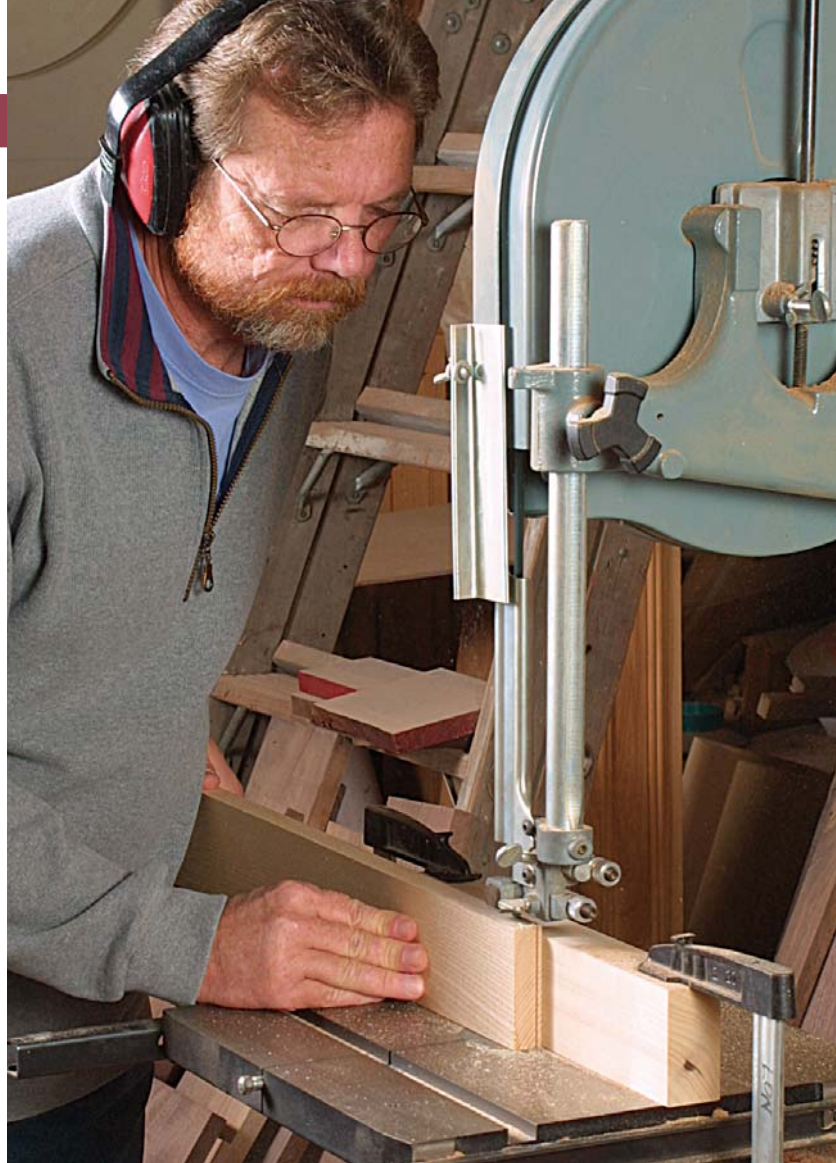
Resaw thick stock for the plies. With the ply stock cut to rough width and length, use a bandsaw to resaw each ply to a thickness that's slightly oversize.
