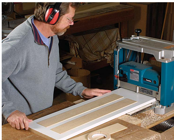
Plane the plies to thickness. Use double-sided tape to secure several resawn surfaces, face up, to a piece of melamine. After a few light passes through a portable thickness planer, the resawn surface ends up smooth, and the plies are reduced to the correct thickness.
