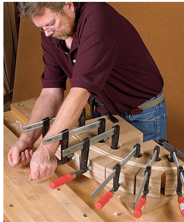
Tighten the clamps. After adding the final clamp, give them all a final check for tightness.
