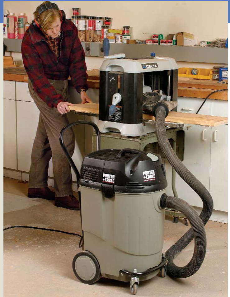
The shop vacuum also serves as a portable dust collector. Depending on the shop, it may be the only means of dust collection or it may be a backup to a larger system.
