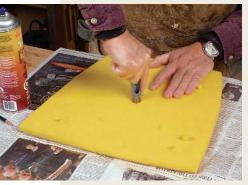
Punch five holes for air to escape. Align these with the slots in the plywood platform below.
