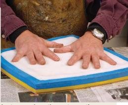
Last, press down the center section. Working from the edges toward the center, compress the softer, oversize center section as evenly as possible.
