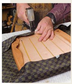
stery fabric the same way. The two tabs of white tape indicate the alignment of the stripes.
