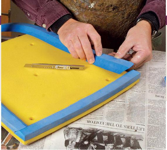
Cut the outer band of foam. Angle the bandsaw table to cut two beveled pieces from a single strip. Apply it flush with the outside edges of the platform, beveling the ends for neat joints.
