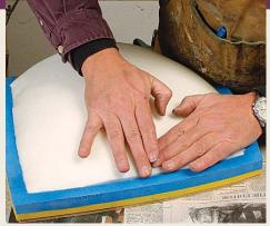
Work in toward the middle of each edge. Be careful to mate each square edge of the center section as smoothly as possible with the beveled edge of the outer band.
