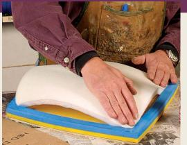
**Start at the corners.** Using spray adhesive on all of the mating surfaces, attach the corners of the center section of medium-density foam to the corners of the high-density outer band.
