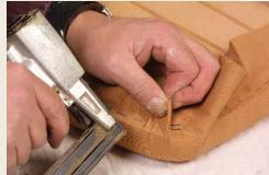
Work toward the corners, a few staples at a time. When you are near the end of an edge, skip ahead to the corner before doubling back to fill in the staples between. This should help you avoid deep wrinkles.
