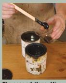
**The second glaze.** Mix raw-umber and black shading and glazing stain thinned with mineral spirits. Brush on the mixture and wipe it off. Residue left in crevices imitates an antique look (right).
