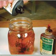
**Combination dye and seal.** This 2-lb. cut of premixed blond shellac is diluted with an equal volume of denatured alcohol (left). A few drops of concentrated dye give this washcoat some color (above).
