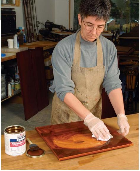
**A second layer of color.** Brush on a shading and glazing stain, then wipe it off. Leave a thin layer of color with a little extra glaze in the corners and voids to give a more interesting look to the piece.
