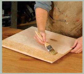
First finish layer. Brush on the dyed shellac. This layer also seals the wood from the next glaze (below).
