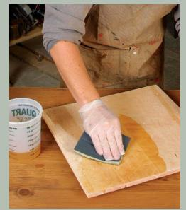
**Fill the eyes and smooth the surface.** Pour a generous amount of the mixture onto the wood and then sand it in with a 400-grit sanding sponge. The oil-and-sawdust slurry fills voids in the bird's eyes, making them more prominent.
