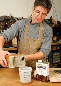
**Create a penetrating oil.** Mix equal amounts of Danish oil and mineral spirits. To avoid spills when pouring, keep the opening at the top to allow air to enter and liquid to exit smoothly rather than in irregular gulps.
