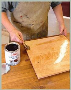
**Topcoat with a clear finish.** To avoid adding a tone to the natural-looking wood, use a nonyellowing finish, such as Behlen's Water White Restoration Varnish.
