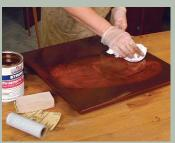
The first glaze. Apply burntumber shading and glazing stain to the sanded shellac. Allow it to penetrate, then wipe the surface, leaving residue in any voids.
