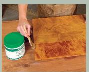
**Dye, then seal.** Apply a waterbased dye (left). When it's dry, seal it with a coat of dark dewaxed shellac, such as buttonlac.
