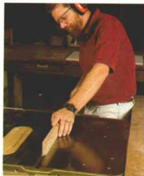
A perfect fit—Runner stock should slide freely in the miter slots (above). Finished runners should be just below the level of the table (right).
