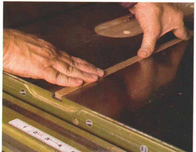
A perfect fit—Runner stock should slide freely in the miter slots (above). Finished runners should be just below the level of the table (right).
