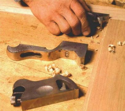
From rabbet plane to chisel plane—Allfour of the Stanley shoulder planes can be converted to chisel planes by removing the nose pieces, allowing the plane to cut right into a corner.
