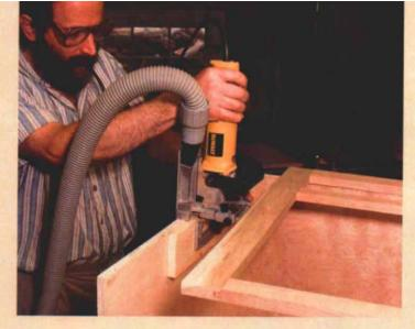
Clamp-up is a cinch with the carcase on its back. Face frames attached with biscuits need to be clamped. Sawhorses make it easy to reach all the edges of the carcase and face frame.
