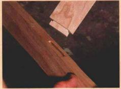
Use mortise-and-tenon joinery for a strong, easily aligned joint. To save time, cut the tenon shoulders on the tablesaw without changing the blade height.
