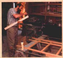
Before glue-up, dry-fit the whole frame. This ensures all pieces will go together smoothly when coping with glue that sets quickly and an armload of clamps.
