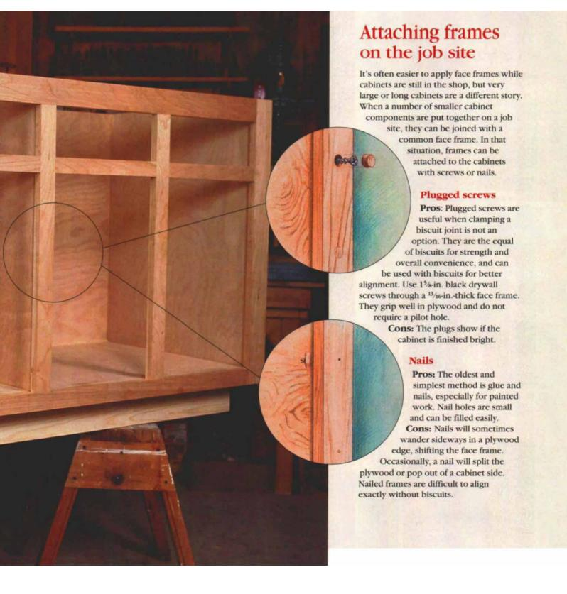
add a clamp across the long diagonal to pull it into place. Despite every care, the square of the door and drawer openings on a complex face frame may not agree with the overall squareness of the frame. When this happens, I split the difference.
