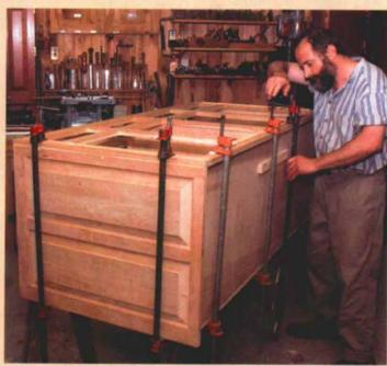
cabinets should be set in place individually, then fastened together to ensure they're square, plumb and aligned.
