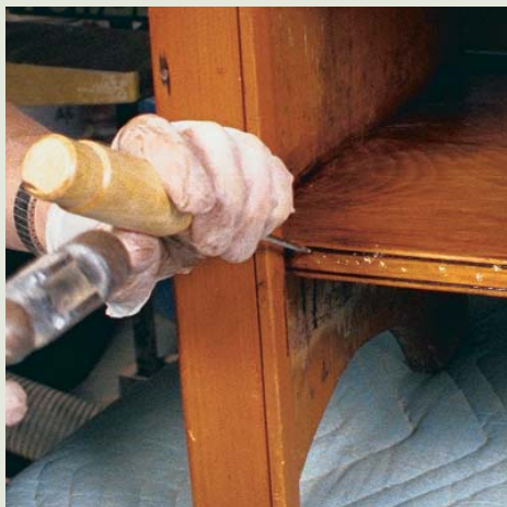
Counterfeit wormholes—After applying a shellac finish but before the final coat of dark, tinted wax, the author uses a small drill bit and the point of an awl to match damage done by worms.
