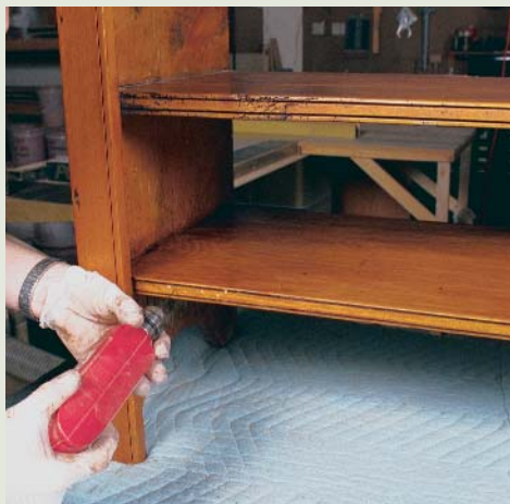
Counterfeit wormholes—After applying a shellac finish but before the final coat of dark, tinted wax, the author uses a small drill bit and the point of an awl to match damage done by worms.
