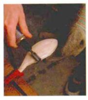
A carbide burr roughs out a spoon blank in no time. Burrs grind wood more than they cut it. This makes them easy to handle for freehand shaping. Wear gloves: If you ever touch a spinning bit, you'll know why. gins to collect, and wipe it off (but not on your shirt).
