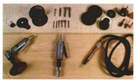
**Grinders for virtually any job**—Air-powered die grinders are an unlikely ally in the woodshop, excelling at jobs like evening up chair legs (right). The author's arsenal includes (from left) an angle grinder, straight grinder, microgrinder and a variety of abrasive discs, wheels and burrs.
