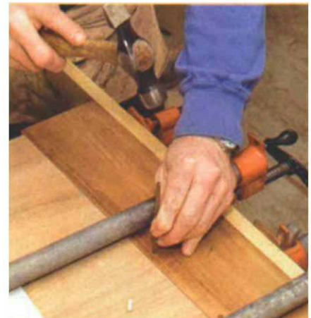
Glue only the center. The center two mortise-and-tenon joints are glued. The other two are pinned through elongated holes but assembled without glue so the top can move with seasonal changes in humidity.
