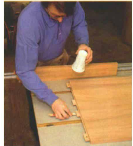
Glue only the center. The center two mortise-and-tenon joints are glued. The other two are pinned through elongated holes but assembled without glue so the top can move with seasonal changes in humidity.
